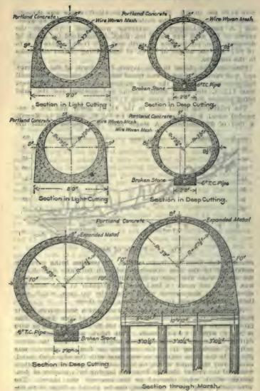
Fig. 18.—Cross Sections of Concrete Sewer.
